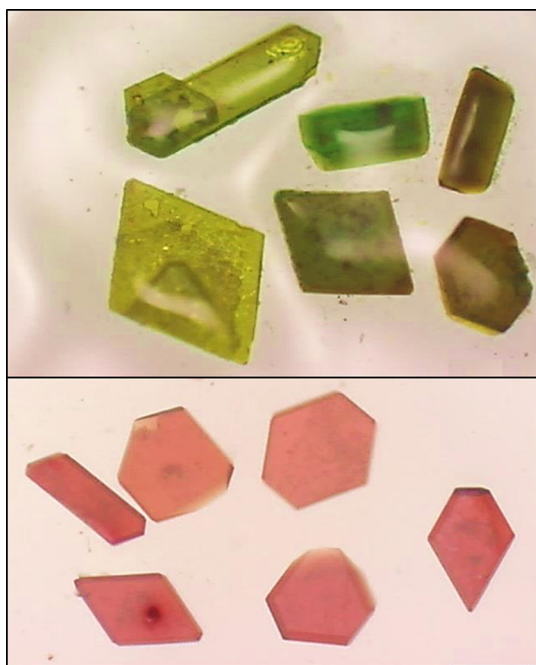
Figure 2. Green crystals of \text{W}_2\text{Cl}_4(\text{OEt})_4(\text{EtOH})_2 and red crystals of \text{W}_2\text{Cl}_4(\text{OEt})_6 from reactions of \text{FeW}_2\text{Cl}_{10} in ethanol.
